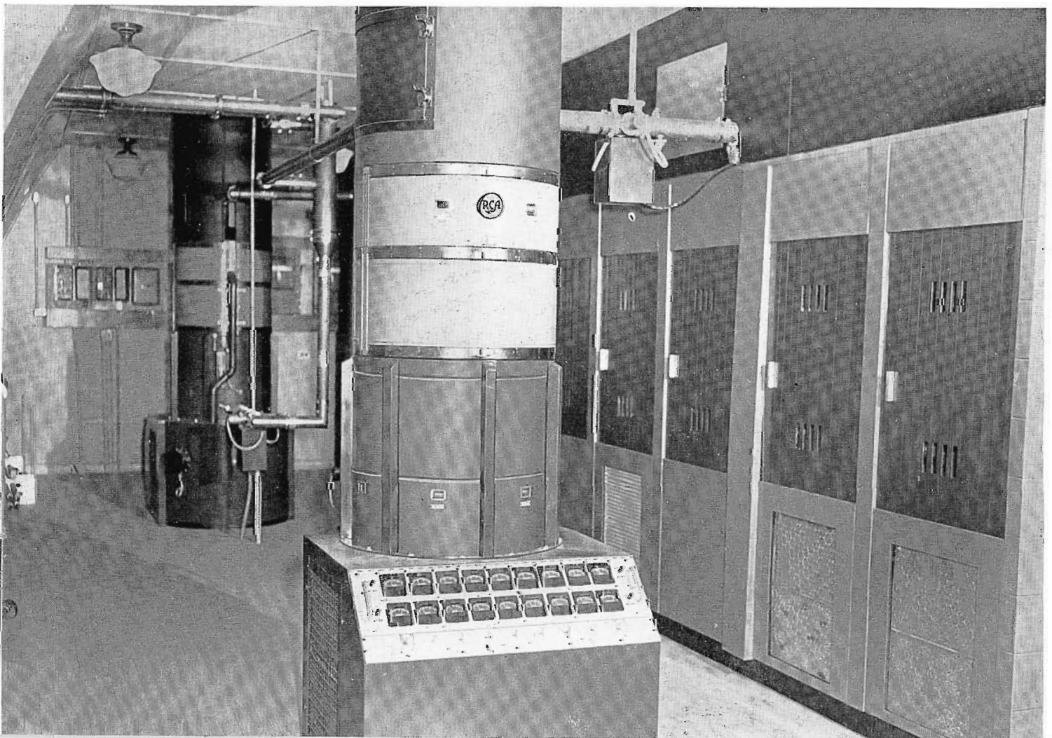
FIG. 6. Shown is a front view of the KBTB 25-KW Aural Power amplifier.
