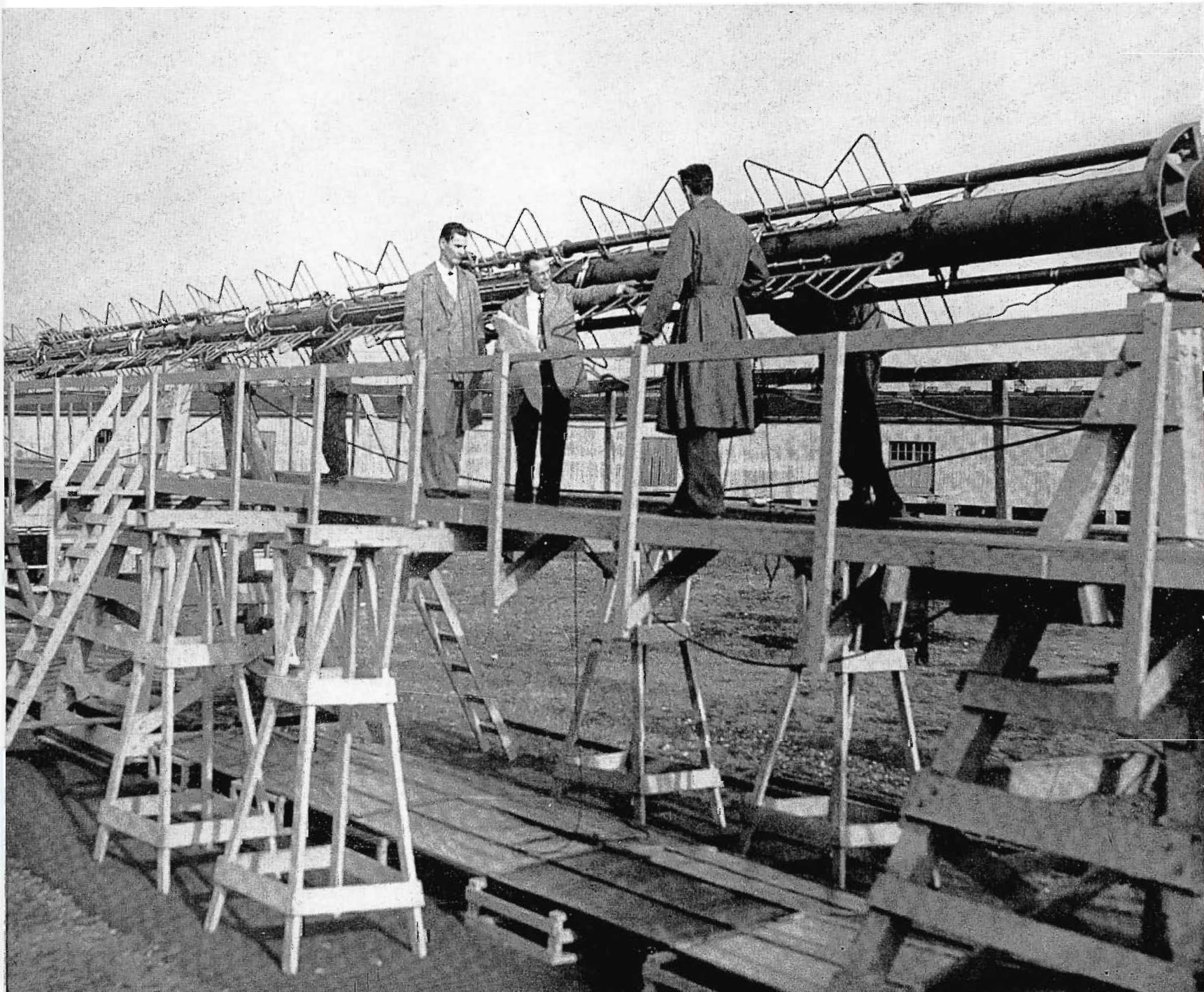
FIG. 1 (below). View of the new 50 KW TF-12BH Superturnstile shown during field tests (space cloth is visible under platform). From left to right: I. T. Newton of Antenna Planning, with M. R. Johns and H. H. Westcott (back to camera) of the Broadcast Antenna Engineering Group.
