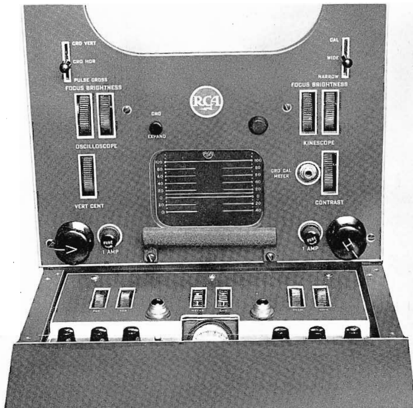
FIG. 9. Closeup view of the Vidicon Camera control unit and the remote control panel which is mounted in the sloping section of the console.
