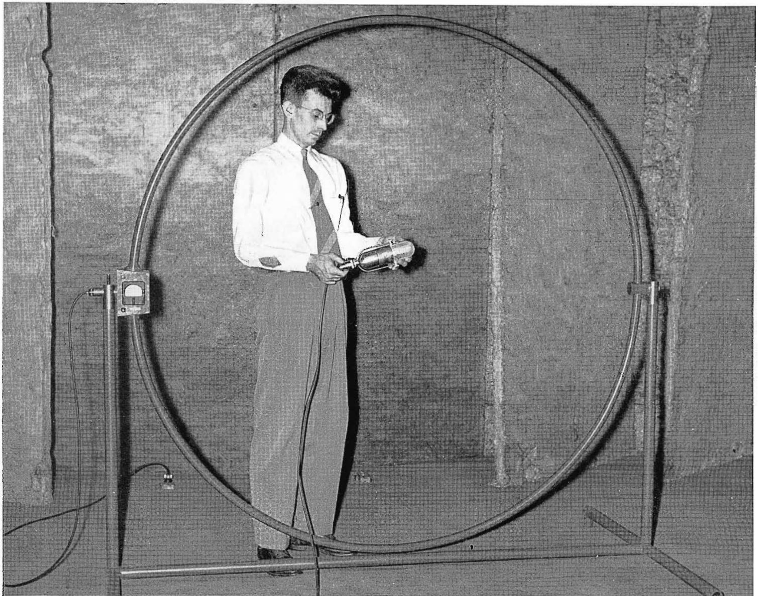
FIG. 1. Sensitivity tests are performed on RCA Type 77-D Polydirectional Microphone by employing field intensity measurements.
