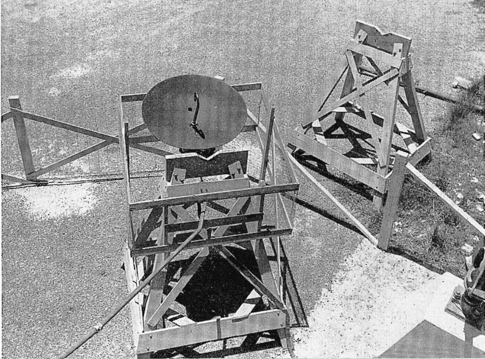
FIG. 6. Microwave relay receiver "dish" at base of tower which delivers signal to transmitter.
