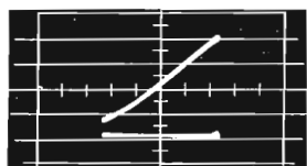
Another linearity trace (taken directly from an oscilloscope) of the TTU-12A when driving the TTU-12A to 12 KW "peak-of-sync" "P.A." output.
