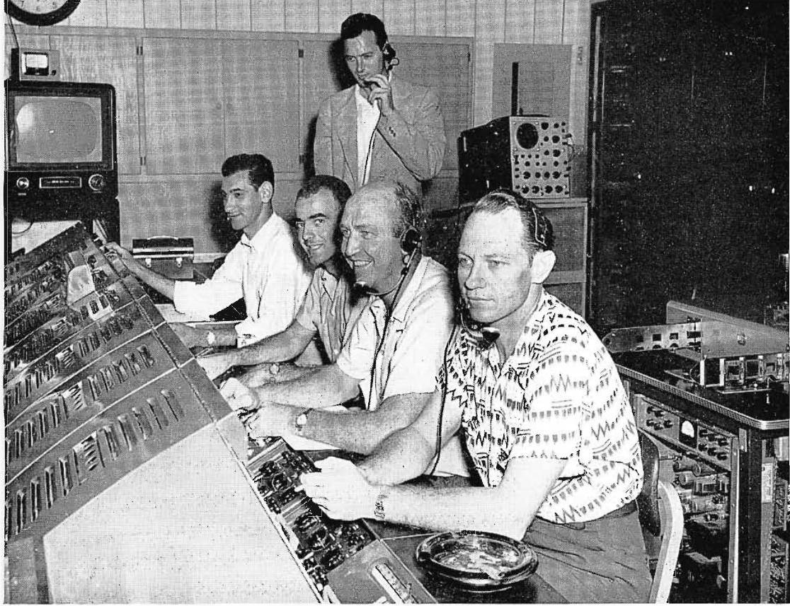
FIG. 4 (above). Master control in operation at WFTL-TV. This bank of RCA monitors, switching and control equipment faces main arena studio.
