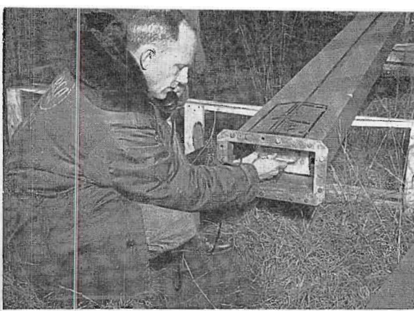
FIG. 2. F. J. McMenam adjusts temporary shorting plate at end of a test length of waveguide (shown below, Fig. 3) for product development test.
