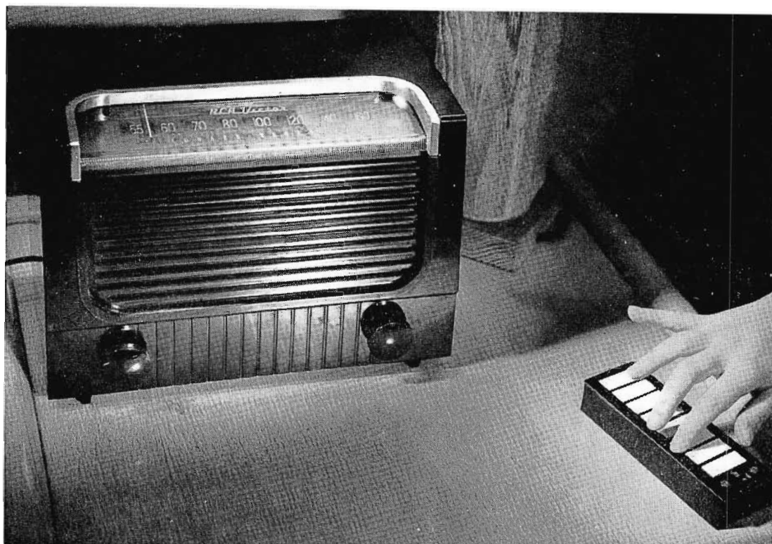
FIG. 8. Toy "piano" operated by one transistor and small battery. This experimental electronic keyboard contains one developmental junction type transistor and eight frequency-selecting circuits—one for each key. Complete scale is produced when "transmitting" to standard broadcast receiver.
