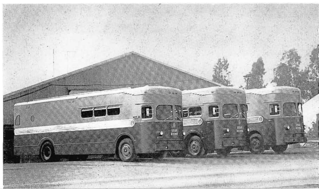
FIG. 2. Complete Television facilities are housed in three 35-foot vehicles of special design.
