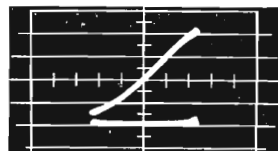
A linearity trace (taken directly from an oscilloscope) of the TTU-12A transmitter at 12 KW "peak-of-sync."
